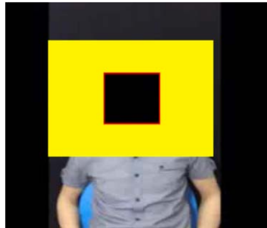
Fig. 6: An example showing the region of the search window with yellow color and this window is used to search for the parts that may appear
