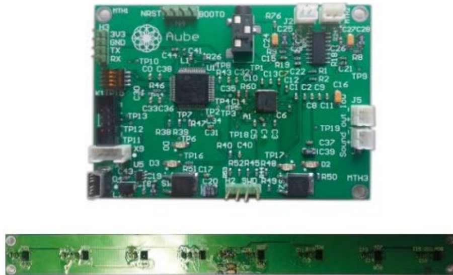
Fig. 2: Linear microphone array used for capturing the dataset and real time experiments with proposed sound source localization
