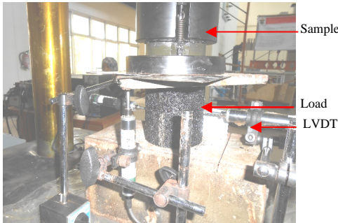
Fig. 4: Setup for the compressive strength test
