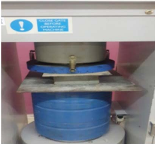
Fig. 3: Bearing strength testing of cementitious brick
