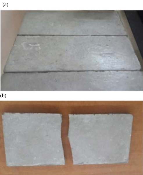
Fig. 7: Cementitious board: a) Self-curing specimens before test and b) After bending test
