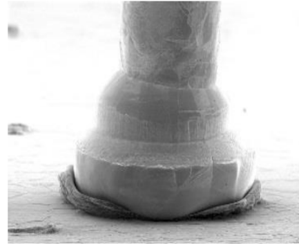
Fig. 13: Bond on high thickness Al bond pad
