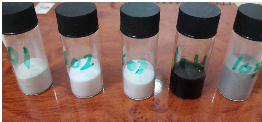
Fig. 1: Silica and hybrid nanocomposite samples were produced: a) CS-SiO 2 ; b) SiO 2 /1; c) SiO 2 /2; d) SiO 2 -MWNTs and e) CS-MWNTs-SiO 2
