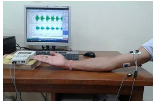
Fig. 2: EMG data acquisition system with the subject
