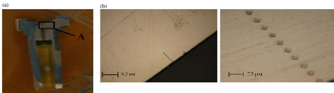
Fig. 9: EHI valve section: a) Filled in epoxy adhesive with subsequent grinding and polishing (actual size) and b) Diamond pyramid traces after microhardening was tested
