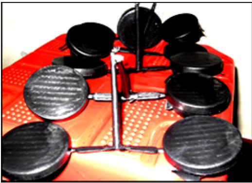
Fig. 7: Some plastic cover products with their nozzle experimentally
