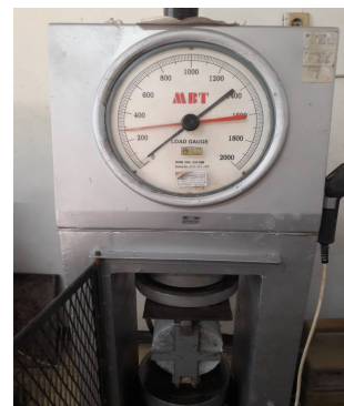
Fig. 2: Set-up of splitting tensile strength test
