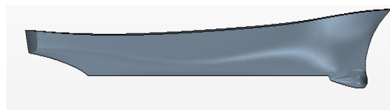
Fig. 1: Geometry of US Navy combatant DTMB
