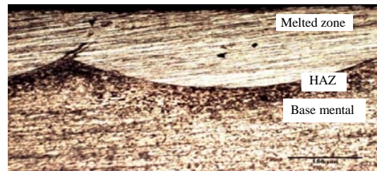
Fig. 2: Laser surface alloying zones within Nickel powder
