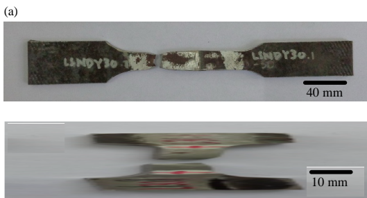
Fig. 12: Fracture of tensile tests; a) Transverse direction and b) Longitudinal direction
