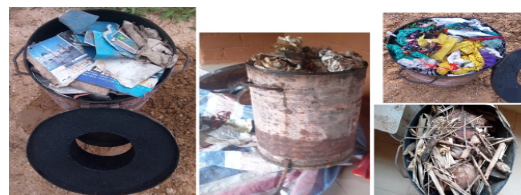
Fig. 1: Filling the carbonizer and pre-closing before firing
