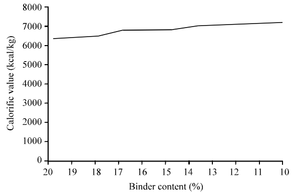
Fig. 15: Evolution of the calorific value of biofuels according to the rate of binder
