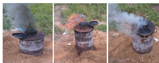
Fig. 2: Control of carbonization and movement of vents
