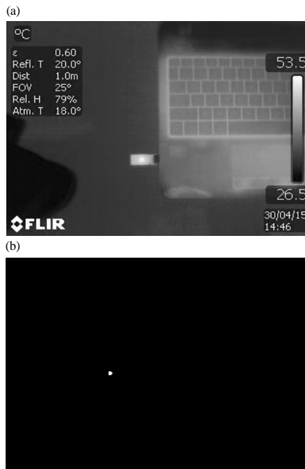
Fig. 4: Image of USB at distance 1 m with emissivity 0.6; a) Grayscale image and b) Output image
