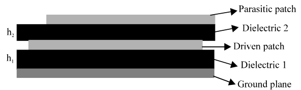
Fig. 3: Side view of proposed stacked antenna
