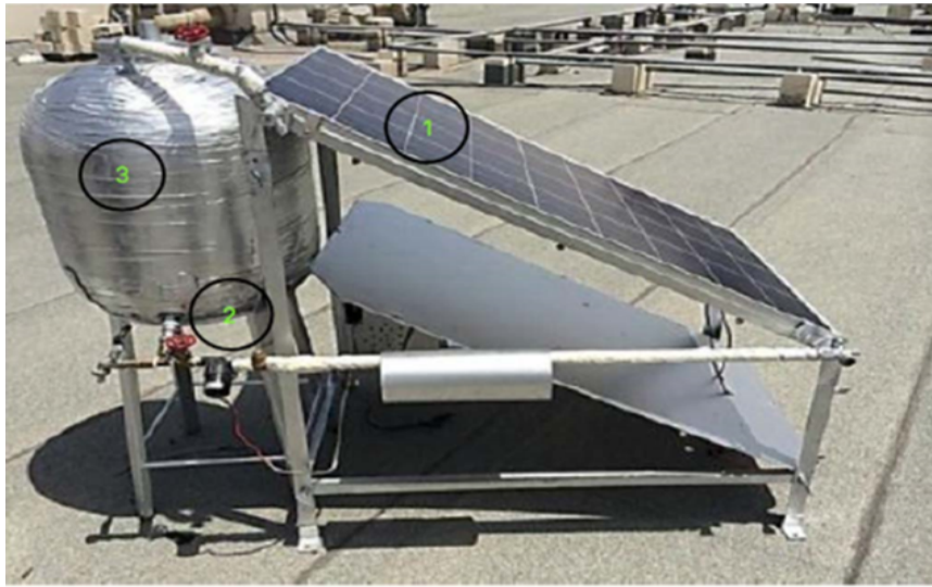
Fig. 5: Hybrid solar Photovoltaic/Thermal (PV-T) cooling by circulation of water (Siecker et al. , 2017)
