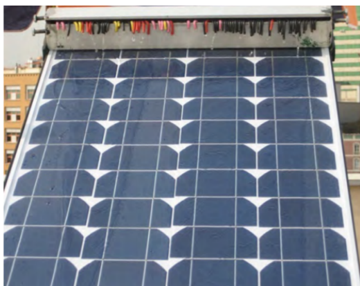
Fig. 4: Solar photovoltaic panel and water film producer equipped with (Hosseini et al. , 2011)
