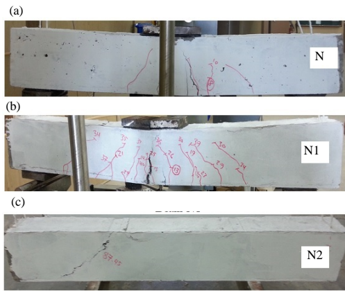
Fig. 5: Crack patterns for voided beams: a) N; b) N1 and c) N2 at ultimate loads
