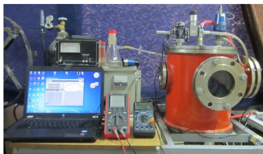
Fig. 3: Gas sensor testing homemade apparatus
