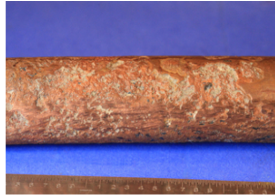
Fig. 6: Stray current corrosion
