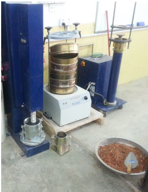
Fig. 4: Compactor apparatus, CBR mold and density mold
