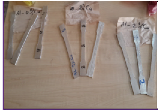
Fig. 5: Tensile test samples of Al-Cu alloy after milling
