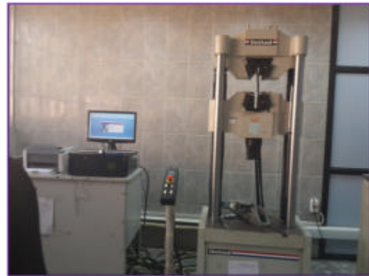
Fig. 6: Tensile test machine used for testing Al-Cu samples
