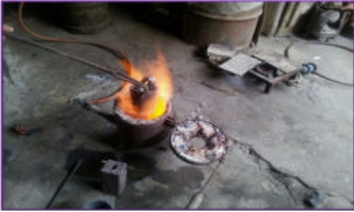
Fig. 2: Melting the aluminium with added copper
