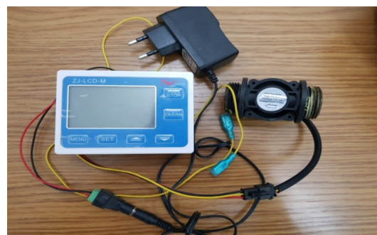
Fig. 6: The digital water flow meter used to measure the water flow rate between cooling tower and heat exchanger
