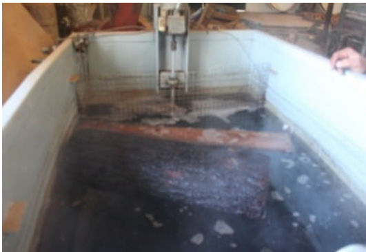
Fig. 10: Steaming operation of the Maritime pine log blocks
