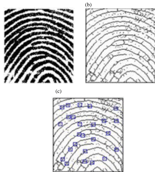
Fig. 2: Steps for minutiae extraction: a) Binary image; b) Thinned image and c) Minutiae of image
