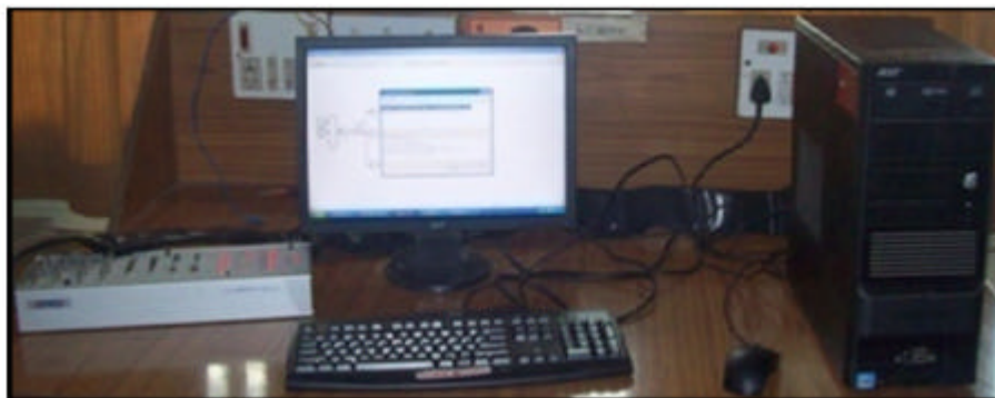
Fig. 16: Experimental setup with DS 1104 in the loop to test the designed digital excitation control system
