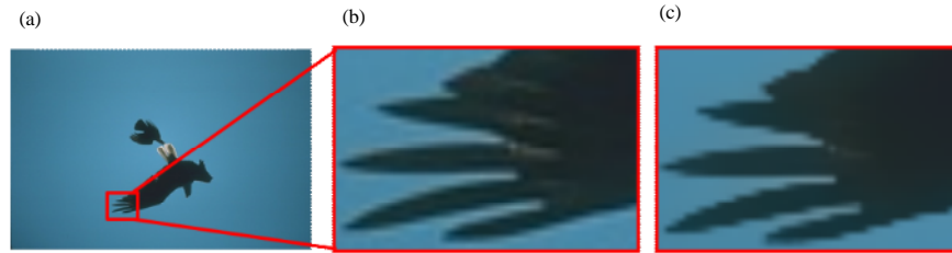
Fig. 1: Bilateral filter: a) Original image; b) Zoom-in original image and c) Zoom-in bilateral filter image
