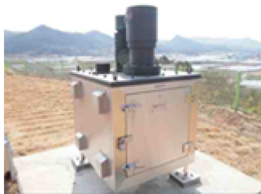
Fig. 1: Automatic cloud observation system
