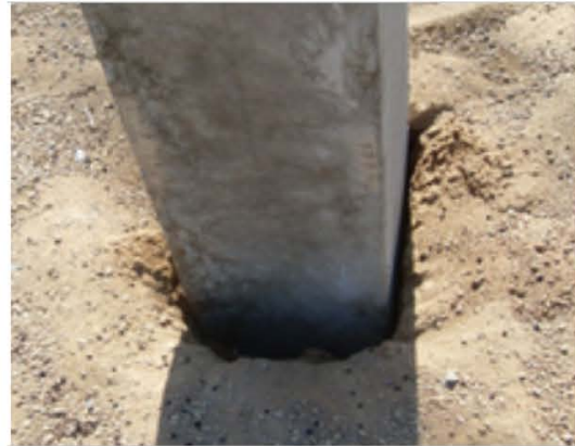
Fig. 1: Gap between sandy soil with rupturing cracks in the corners when the pile body is tilted from misaligned hammer impacts during pile driving
