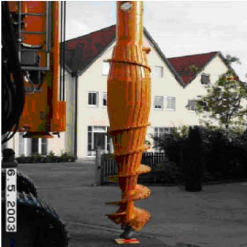
Fig. 16: Bayer displacement drilling system
