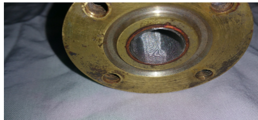
Fig. 2: Wick turn inside heat pipe
