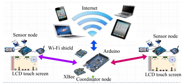
Fig. 1: System architecture of automation of chicken hatchery based on WSN and IoT
