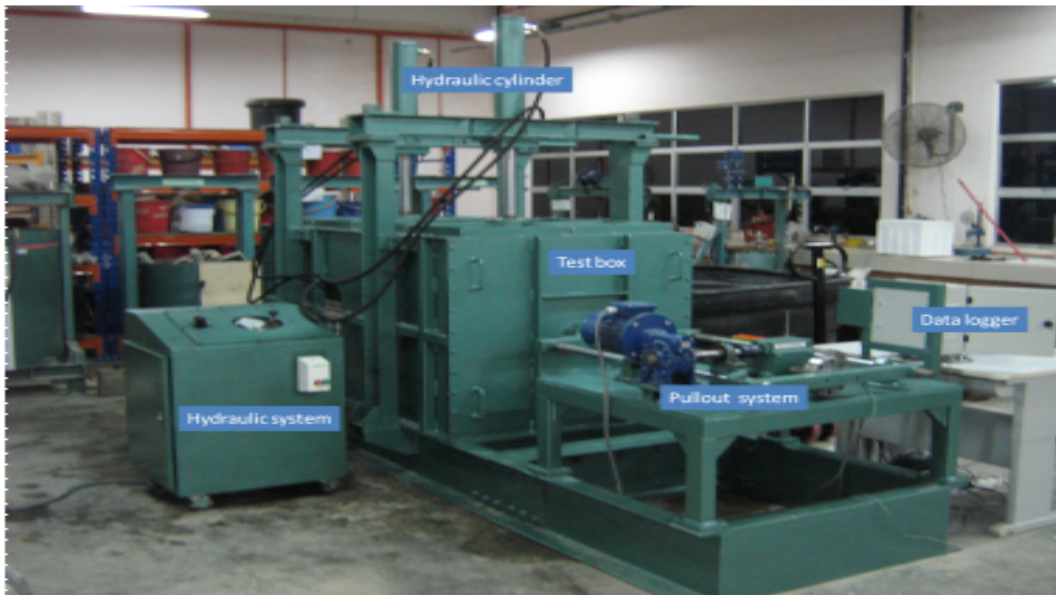
Fig. 12: Pullout apparatus with 3 major components
