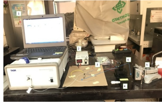
Fig. 1: Experimental setup of FBG pressure sensor, (1) OSA, (2) Laser source, (3) Optical circulator, (4) MMSM, (5) Fixation device and (6) FBG sensor
