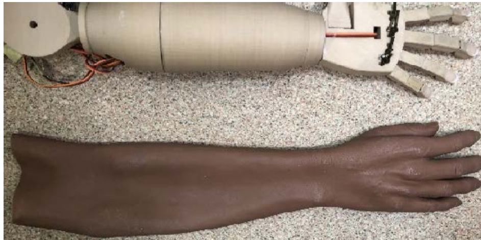
Fig. 4: 3D printed hand with German cosmetic cover for upper limb
