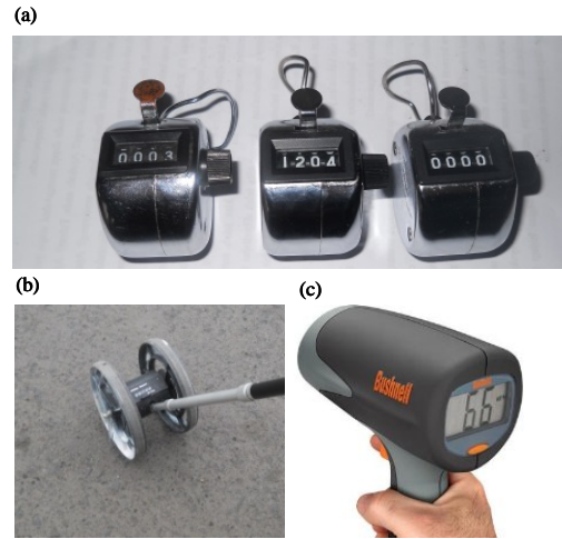
Fig. 8: Instruments used in traffic flow measurement
