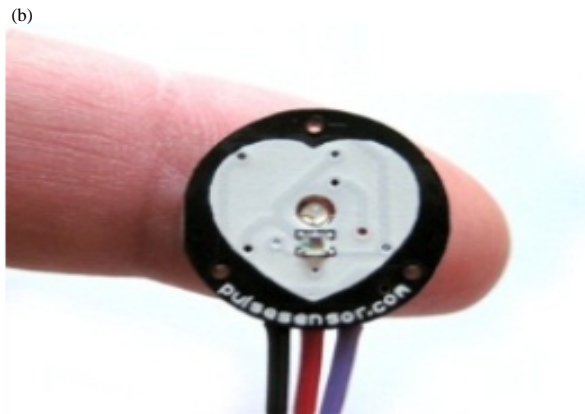
Fig. 2: a, b) Schematic and physical display of pulse sensor circuit
