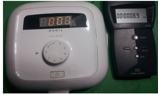
Fig. 9: Prototype and PULSE (HCP03) magnetic field measurement
