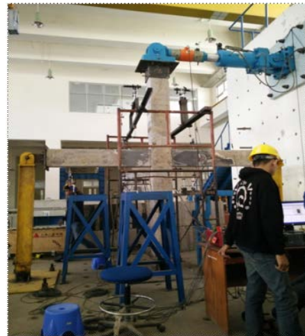
Fig. 12: The cyclic test was used a hidrouic jack, supporters and LVDT
