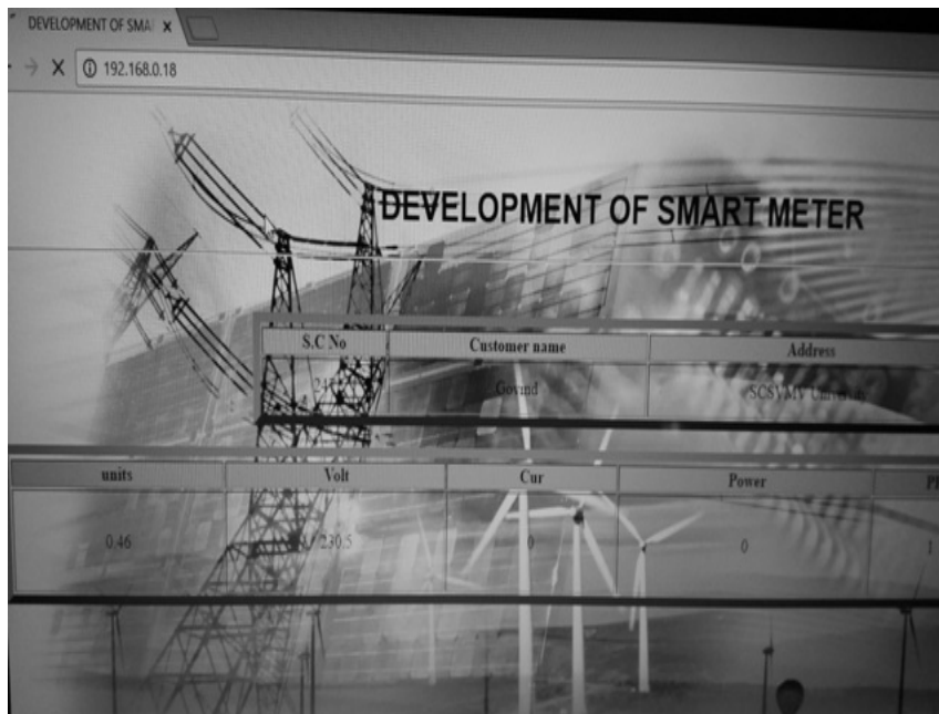
Fig. 8: Web interface for monitoring power consumption
