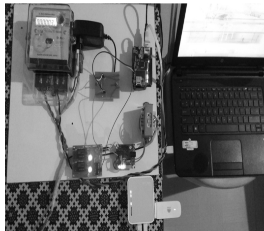
Fig. 6: Monitoring hardware interface
