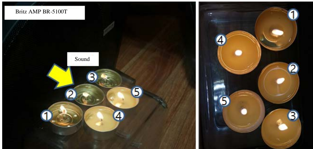
Fig. 3: Experiment scene (measuring the dispersive size of the candlelight)
