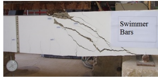
Fig. 13: Typical shear failure
