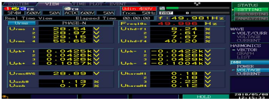
Fig. 41: Experimental results-DVR with SPWM for swell (10%) Total Harmonic Distortion (THD)
