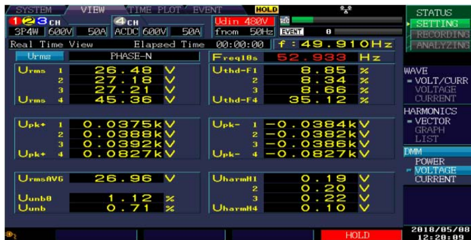
Fig. 45: Experimental results-DVR with SPWM for sag (36%) Total Harmonic Distortion (THD)
