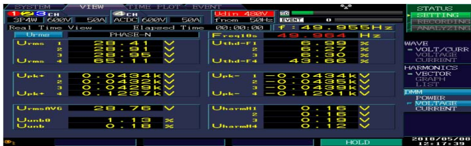
Fig. 36: Experimental results-DVR with SPWM for swell (36%) voltage without compensation
