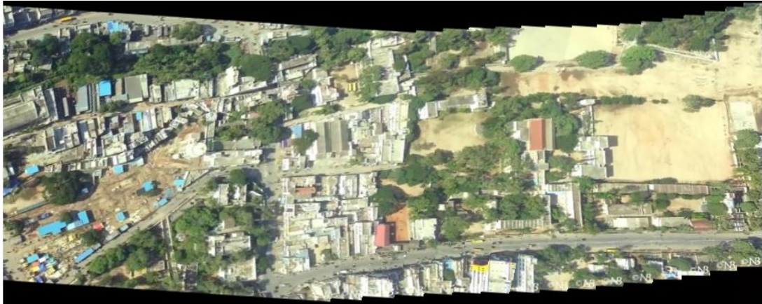
Fig. 10: Mosaic image constructed with only 20 frames out of 627 frames of a video with Intel Compute Stick
