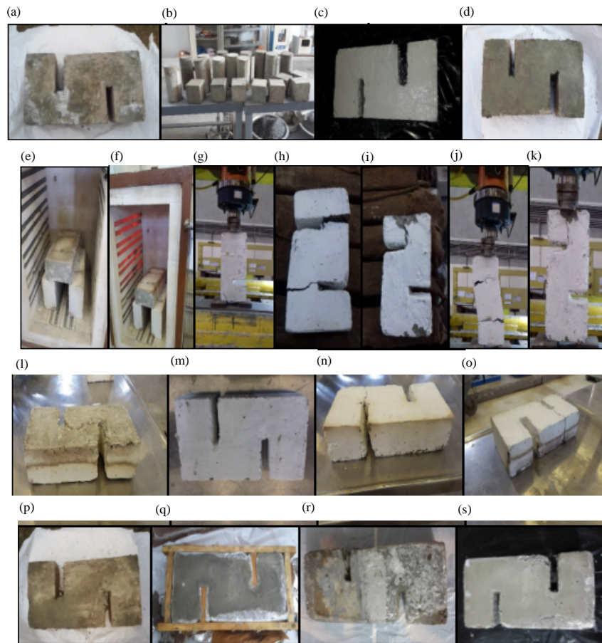
Fig. 16: a-s) Mechanical properties tests and modes of failure and cracking shapes of push-off specimens
