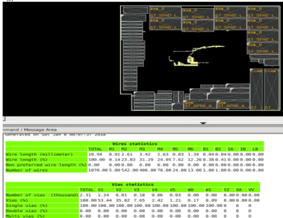
Fig. 3: Nets wire highlighting in the GUI: a) Baseline and b) Proposed flow
