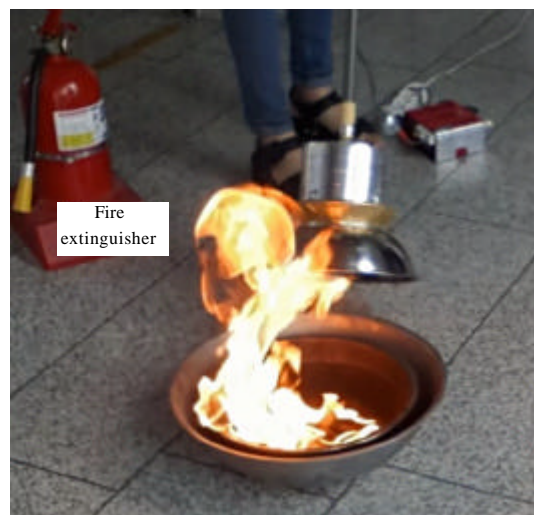
Fig. 1: Sound fire extinguisher
