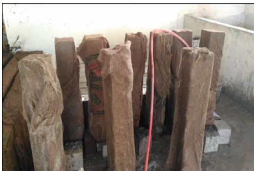
Fig. 6: Curing of specimens
