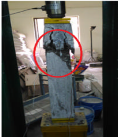
Fig. 10: Crushing failure of column
