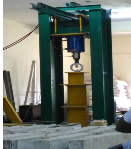
Fig. 7: Column testing machine (100 tons)
