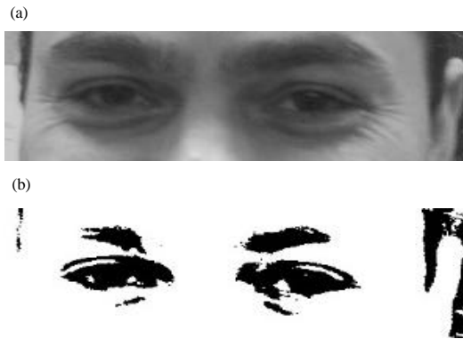
Fig. 2: Eye-lid movement (closed or open) detection converting image to grayscale and binary: a) Greyscale image and b) Binary image with 50-pixel value threshold
