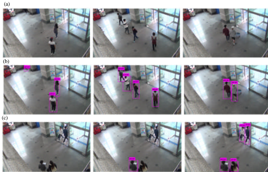
Fig. 6: The original images and the results of human detection using the proposed method: a) The original images; b) Result of human detection using proposed method and c) A comparison of the results between the existing YOLOv2 and the proposed method
