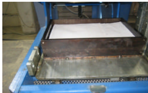
Fig. 14: Compaction of slab by roller compacter
